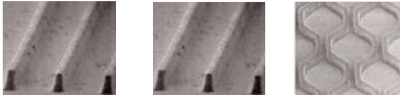
Examples of the barriers that isolate each cell. The distance between the walls of each cell is a couple hundred micrometers – or about ten times the diameter of a human hair (Source: www.plasmacoalition.org )
