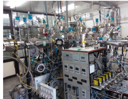
Multiple Magnetron sputtering system for developing solar cell
