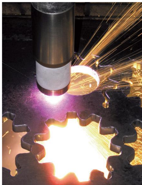
Plasma can be used to cut through metals at high velocity
