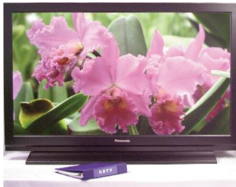
Today's PDP with up to 80" diagonal screens and millions of individual colour elements.
